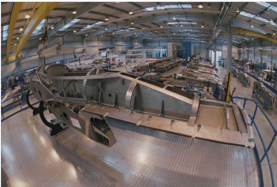
Figure B-2 Pylon Ready to Go
