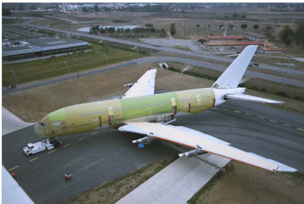
Figure B-4 Empty Pylons
