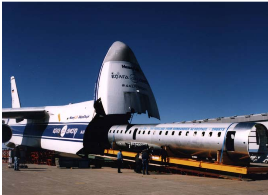
Figure A-12 A Q400 Fuselage Arrives from MHI, Japan
