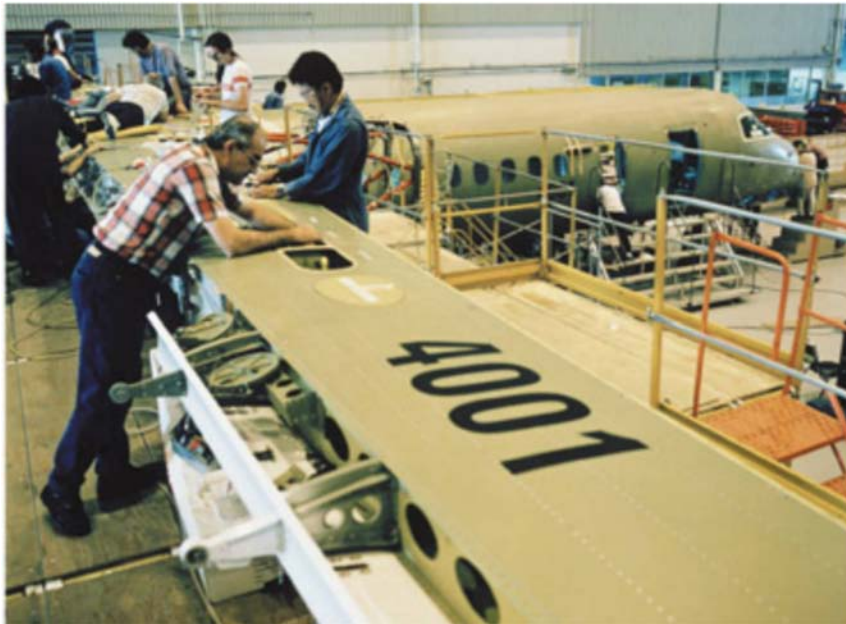
Figure A-5 Bombardier QR 400 Wing Assembly
