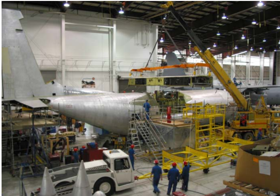
Figure A-1 Rebuilding a C-130 Centre Wing
