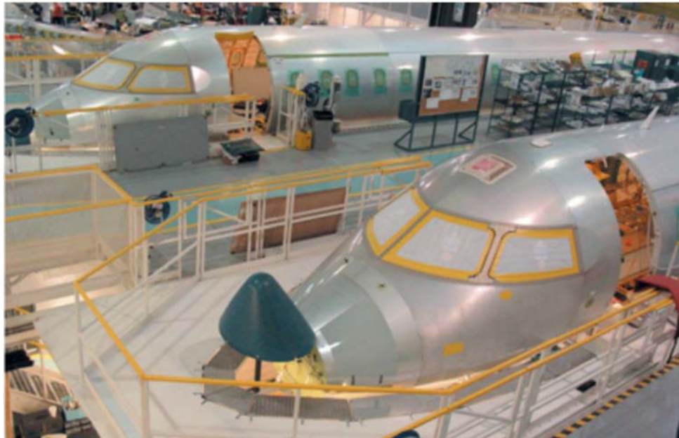
Figure A-9 Bombardier CRJ700 Fuselage Assembly
