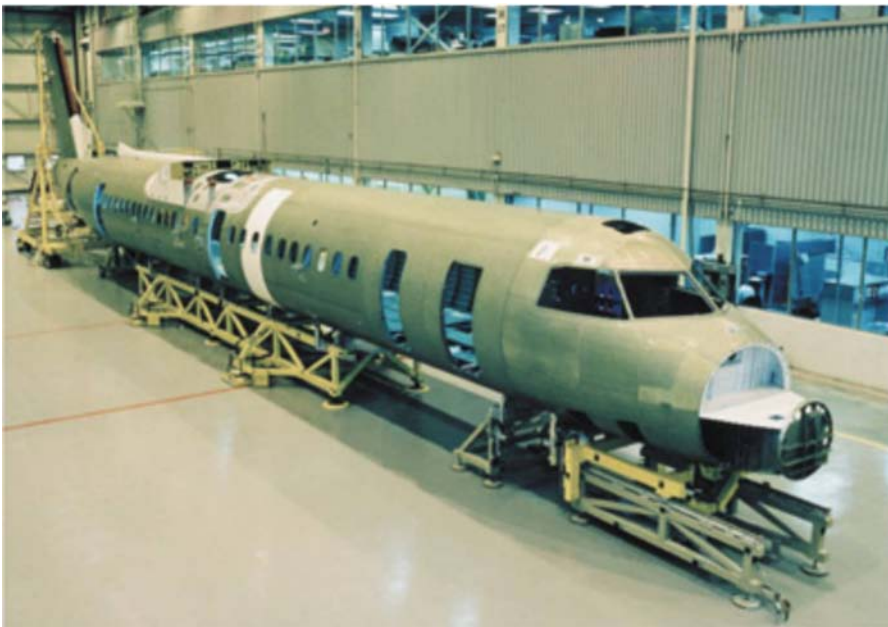
Figure A-4 Bombardier QR 400 Fuselage Assembly
