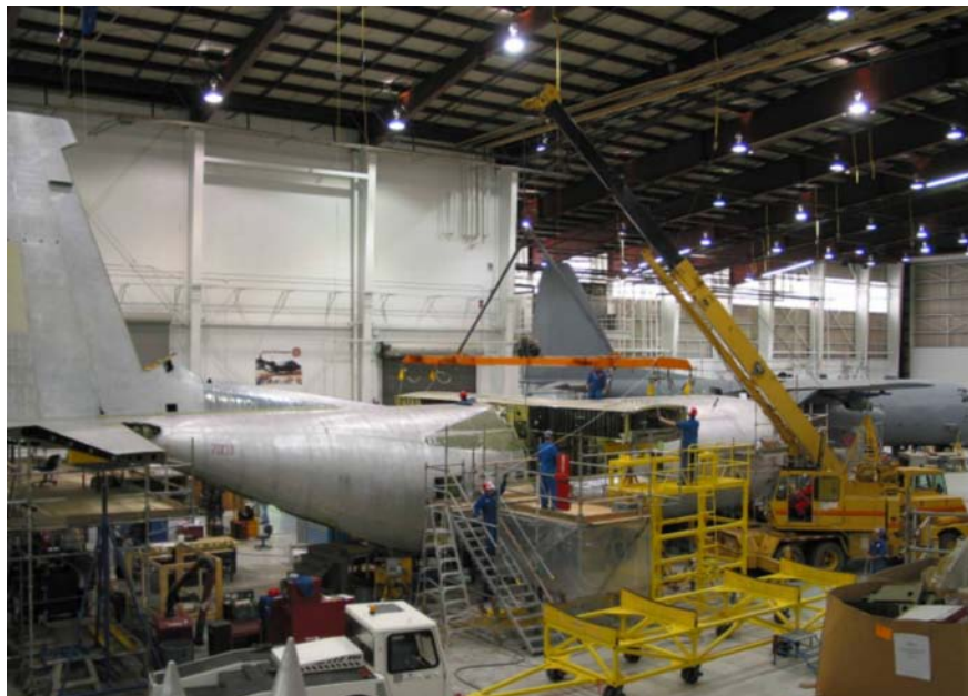
Figure A-2 Placing a C-130 Centre Wing
