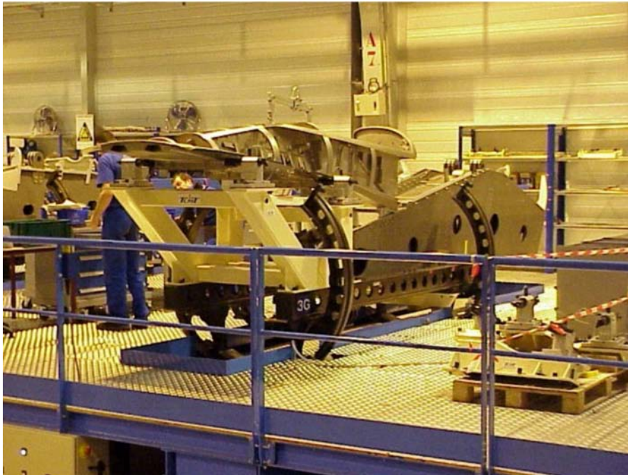
Figure B-1 Building a Pylon
