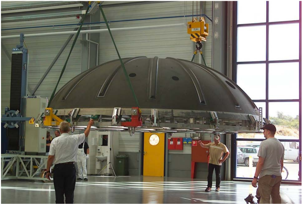
Figure 17O-1 A380 Rear Pressure Bulkhead
