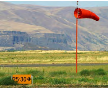
Windssock Indicates the direction and speed of the wind.
