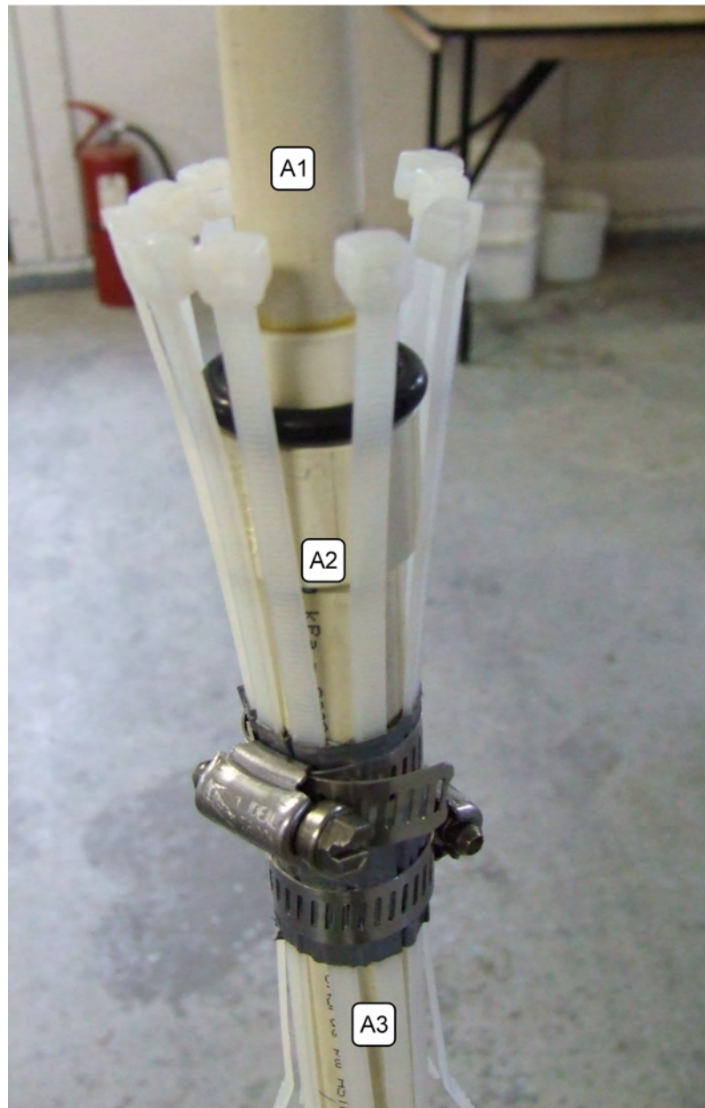
Figure 25-A Tie Cables Clamped to A3
