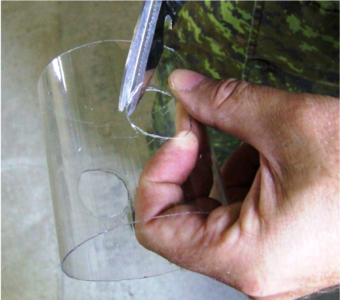
Figure 27-A Cutting the Hole in the Plastic Spring for Section A
