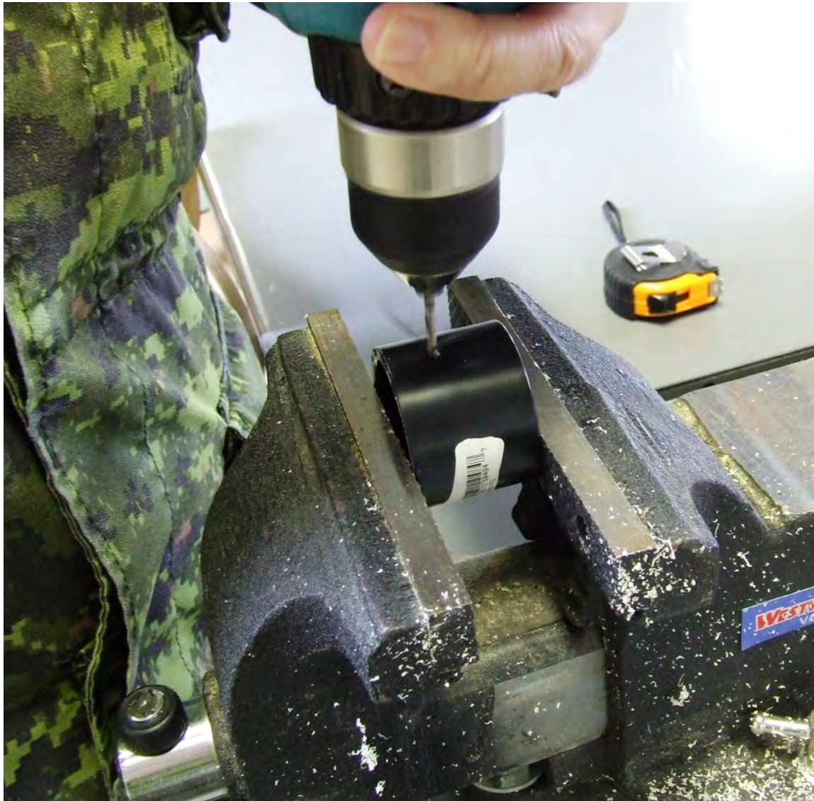
Figure 26-A Drilling 1/8-inch Holes in the ABS Coupler
